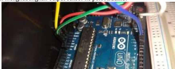
Gambar 12 Pin OUT sensor ke port Arduino
