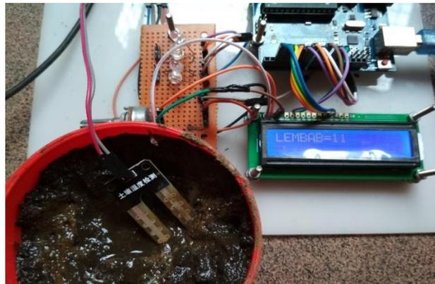
Gambar 9 Pengujian Sensor Soil Moisture FC-28
