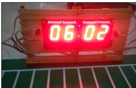
Gambar 10. Pengujian seven segment
