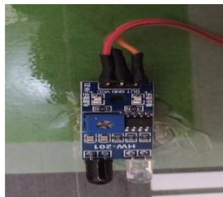
Gambar 7. Sensor Photodioda
