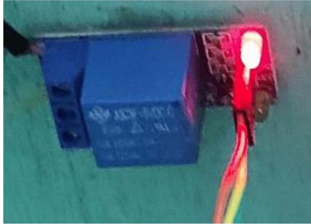
Gambar 5. Tampilan rangkaian relay saklar pompa DC
