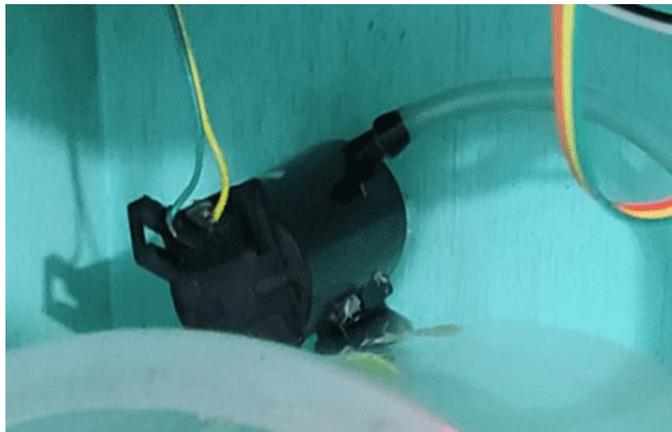
Gambar 7. Pompa air DC
