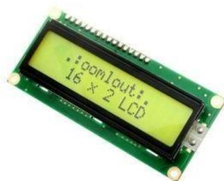
Gambar 7. LCD (*Liquid Crystal Display*)
